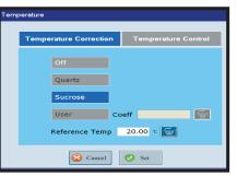
(3) A Quartz Plate measured at 25°C by the chamber temperature probe can be automatically corrected to 20°C.
